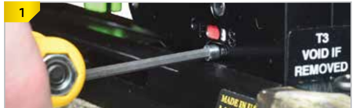
Remove the hex-head cap screw.
