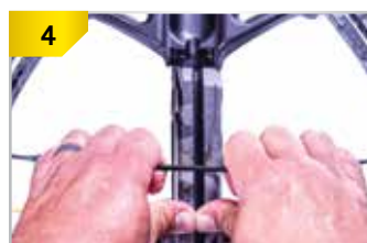
Pull up and back slightly on the bowstring to seat the bow assembly.
