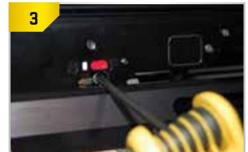
Re-insert the hex-head cap screw into the safety knob.
