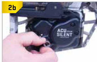
2b Loosen the silver crank collar until it stops.
