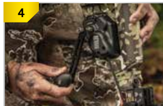
Turn the crank handle counter-clockwise (backwind) until the bowstring is lowered to its resting/relaxed position.
