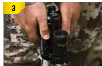
Align the magnets from the T-handles with the magnets on the sled.
