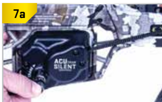
7a Remove crank handle.
