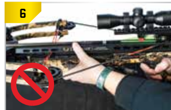
IMPROPER HAND POSITION. With your fore-grip hand rotated to the side of the grip, you will expose your thumb to the bowstring's release path.
