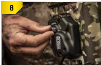
Turn the crank collar forward, finger tight only.
