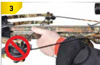
IMPROPER HAND POSITION. With your fore-grip hand positioned as shown above, you will severely injure your hand or amputate your thumb and/or finger(s) if you fire your crossbow.
