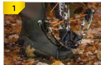
Place your foot firmly inside the foot stirrup.
