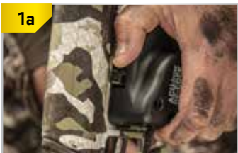
Depress the Gear Stop Button.
