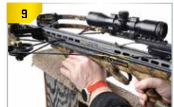
Keep your thumb and fingers below the flight deck and away from the cables to avoid injury.
