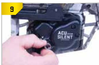
9 Turn collar forward to keep claw from moving.
