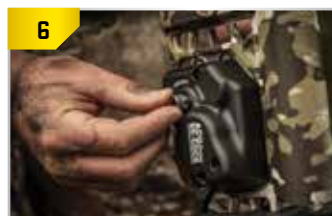
Use your fingers to turn the crank collar counter-clockwise (backward) until it stops.
