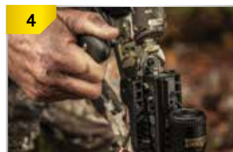
Turn crank handle clock-wise (forward) until the safety button pops out.
