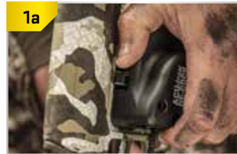
Depress the Gear Stop Button.
