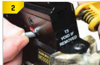
Insert aluminum safety knob.
