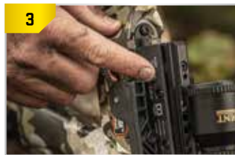
Depress the De-Cock Button, then insert the crank handle and turn 1 - 1 1/2 full turns forward.
