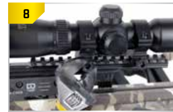
Determine scope position and tighten the scope nuts onto the dovetail mount.
