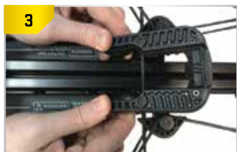
Connect the string slots to the bowstring and lower the guidepost into the barrel's flight groove.
