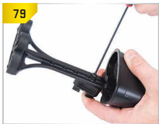
Use a 5/64-inch Allen wrench to remove/reinsert the mounting block button head cap screw.
