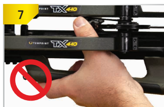
7 IMPROPER HAND POSITION. With your fore-grip hand positioned as shown, you will severely injure or amputate your thumb if you fire your crossbow.
