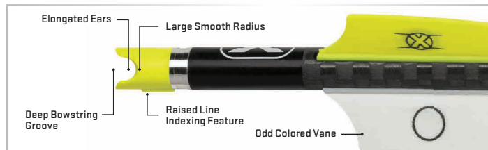
Correct Alpha-Nock HP/HPX Orientation
