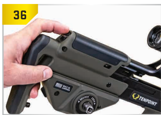
Press trigger release-latch.
