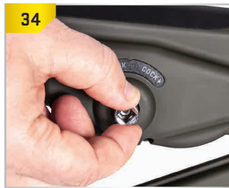
Backwind the silver collar one (1) complete turn by hand or until it stops.
