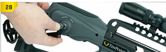
Insert crank handle into the ACUslide's square recess hole.
