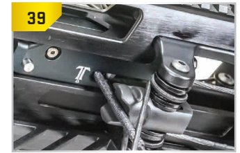
Proper string latch position.
