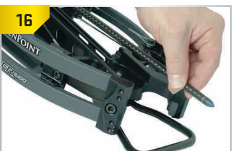
16 PROPER HAND POSITION. Hold the arrow with your index and middle finger and your thumb just behind the broadhead.
