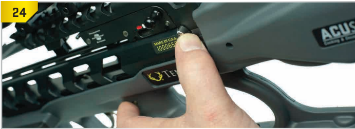
Press trigger box lock-latch lever.
