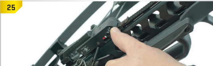
Push down on the forward assist knob.
