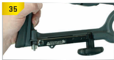
Insert the crank handle into its storage position in the stock.
