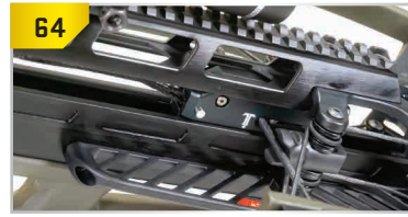
Trigger box attached to the bowstring.
