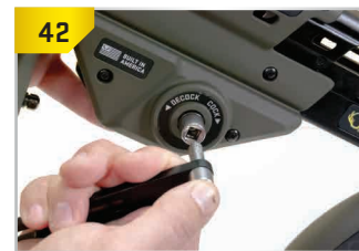
Insert crank handle into the ACUslide Maxx's square recess hole.
