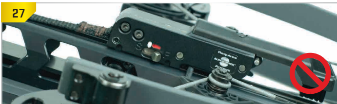
IMPROPER POSITION. String seated on the DFI, safety knob not in the "S" (Safe) position.
