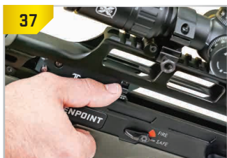
Press down on the forward assist knob.
