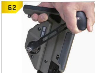
Press the trigger lock-latch down and backwind until the trigger moves 1/2-inch.
