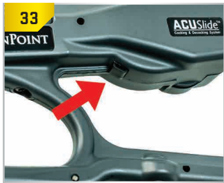
Press in and Hold the Gear Stop Button.
