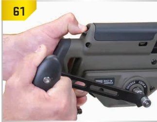
Press trigger release-latch and turn the crank handle forward - just until you remove the tension on the trigger release-latch.
