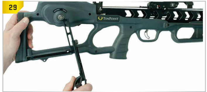
Rotate the crank handle forward to cock the crossbow.
