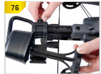
Turn crossbow upside-down, loosen thumb screw, then slide the clamp onto the picatinny rail with the quiver cup facing up.
