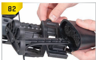
Turn crossbow upside-down, loosen thumb screw, then slide the clamp onto the picatinny rail with the quiver cup facing up.
