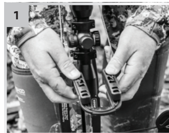
Pull the sled over the scope and attach it to the string.
