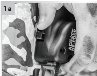
Depress the Gear Stop Button.
