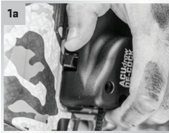
Depress the Gear Stop Button.
