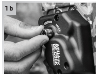
Backwind the crank collar.
