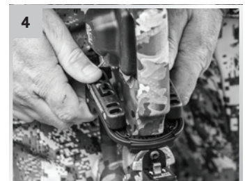
Remove the sled from the bowstring and return it to its storage position on the butt stock.
