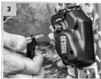
Insert the crank into the crank collar.
