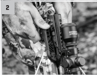
Place the claw securely on the bowstring.
