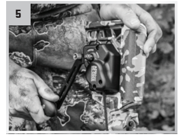
Crank the handle in reverse (counter-clockwise) approximately two to three times.
