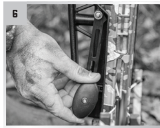
Place the crank handle back in its storage position.
