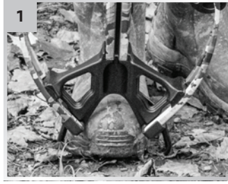
1 Place your foot firmly inside the foot stirrup.
