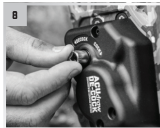
Turn the crank collar forward, finger tight only.
