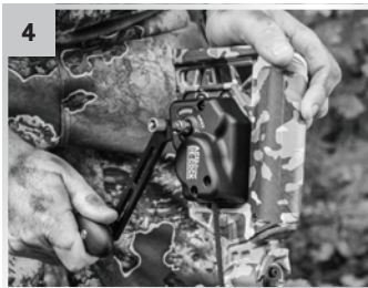
Turn the crank handle counter-clockwise (backwind) until the bowstring is lowered to its resting/relaxed position.
