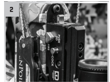
The triangular safety button will pop out when the crossbow is fully cocked.
