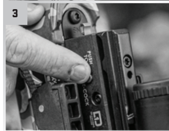
Depress the De-Cock Button, then insert the crank handle and turn 1 - 1 1/2 full turns forward.
