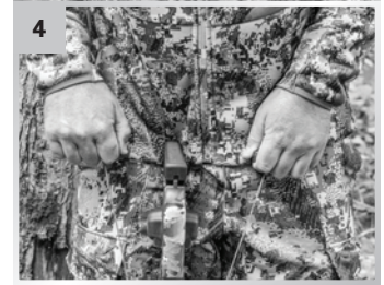
4 Pull up on the T-handles until you hear a click, then you can lower the sled and bowstring.
