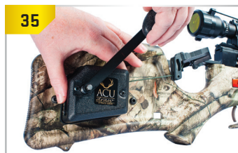
Relieve the tension on the ACUdraw device before lifting the claw out of its storage position (approximately 1/4-inch to 1/2-inch).
