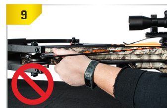
IMPROPER HAND POSITION. With your fore-grip hand positioned in front of the grip, you will expose your thumb to the bowstring's release path.
