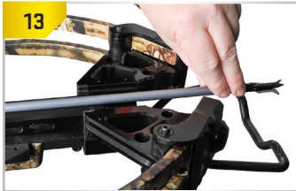
PROPER HAND POSITION. Hold the arrow with your index and middle finger and your thumb just behind the broadhead.
